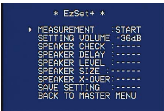
Figure 48 – EzSet+ – Setting Master Volume Level
